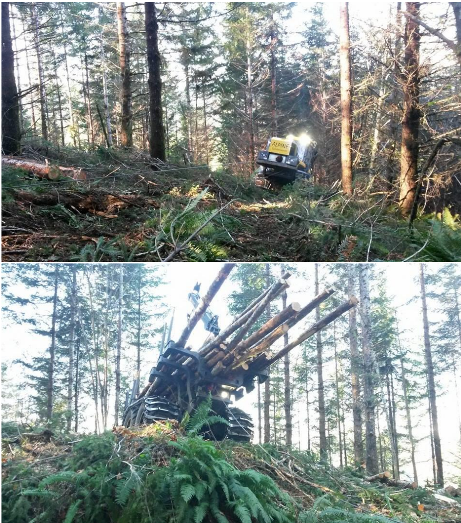
Figure 2.2: Ponsse Bear harvester (above) and Elephant King forwarder (below) on tethered thinning operations in the Oregon Coast Range
